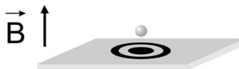
Fig. 1. Conceptual view of a planar trap with two electrodes. For negatively charged particles, the disk electrode must have a potential smaller than the ring electrode.
